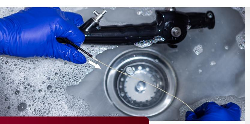
Designed to be backloaded through the working channel. (insert brushless end into the luer connector, and remove from the distal end of the scope).
